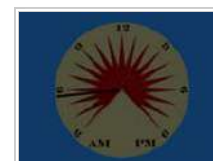
Top view of an equatorial sundial. The hour lines are spaced equally about the circle, and the shadow of the gnomon (a thin cylindrical rod) rotates uniformly. The height of the gnomon is 5/12 the outer radius of the dial. This animation depicts the motion of the shadow from 3 a.m. to 9 p.m. (not accounting for Daylight Saving Time) on or around Solstice, when the sun is at its highest declination (roughly 23.5°). Sunrise and sunset occur at 3am and 9pm, respectively, on that day at geographical latitudes near 57.05°, roughly the latitude of Aberdeen, Scotland or Sitka, Alaska.
