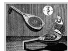
Diptych sundial in the form of a lute, c. 1612. The gnomons-style is a string stretched between a horizontal and vertical face. This sundial also has a small nodus (a bead on the string) that tells time on the hyperbolic pelikonon , just above the date on the vertical face.
