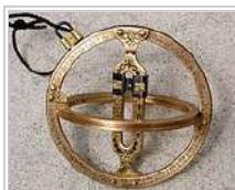
Universal ring dial. The dial is suspended from the cord shown in the upper left; the suspension point on the vertical meridian ring can be changed to match the local latitude. The center bar is twisted until a sunray passes through the small hole and falls on the horizontal equatorial ring.
