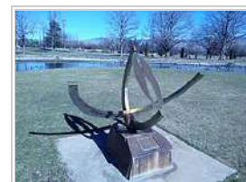
A combined analemmatic-equatorial sundial in Ann Morrison Park in Boise, Idaho, 43°36'45.5"N 116°13'27.6"W
