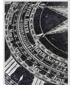
The Whitehurst & Son sundial made in 1812, with a circular scale showing the equation of time correction. This is now on display in the Derby Museum.
