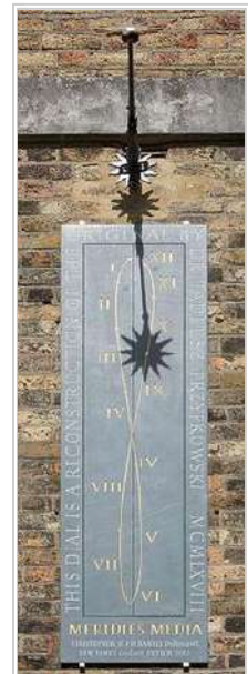
Noon mark from the Greenwich Royal Observatory. The analemma is the narrow figure-8 shape, which plots the equation of time (in degrees, not time, 1° =4 minutes) versus the altitude of the sun at noon at the sundial's location. The altitude is measured vertically, the equation of time horizontally.
