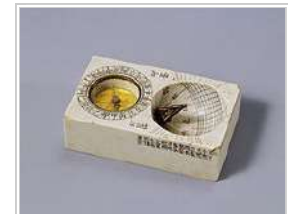
Angbuilgu , a portable sundial used in Korea during the Joseon period. The integrated magnetic compass aligns the instrument toward north pole. (National Museum of Korea) [81]
