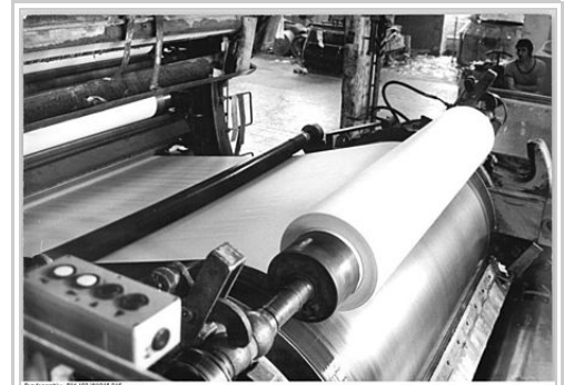
Paper leaving the machine is rolled onto a reel for further processing.
