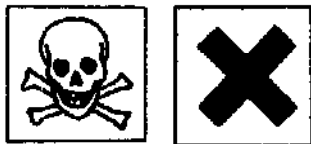
Figure 6.9. Two warning signs often used on labels of chemicals to express acute toxicity. The skull indicates a toxicity by which 0.3 grams of the chemical are lethal, an St. Andrew's cross indicates a fatal toxicity of 3.30 grams.
