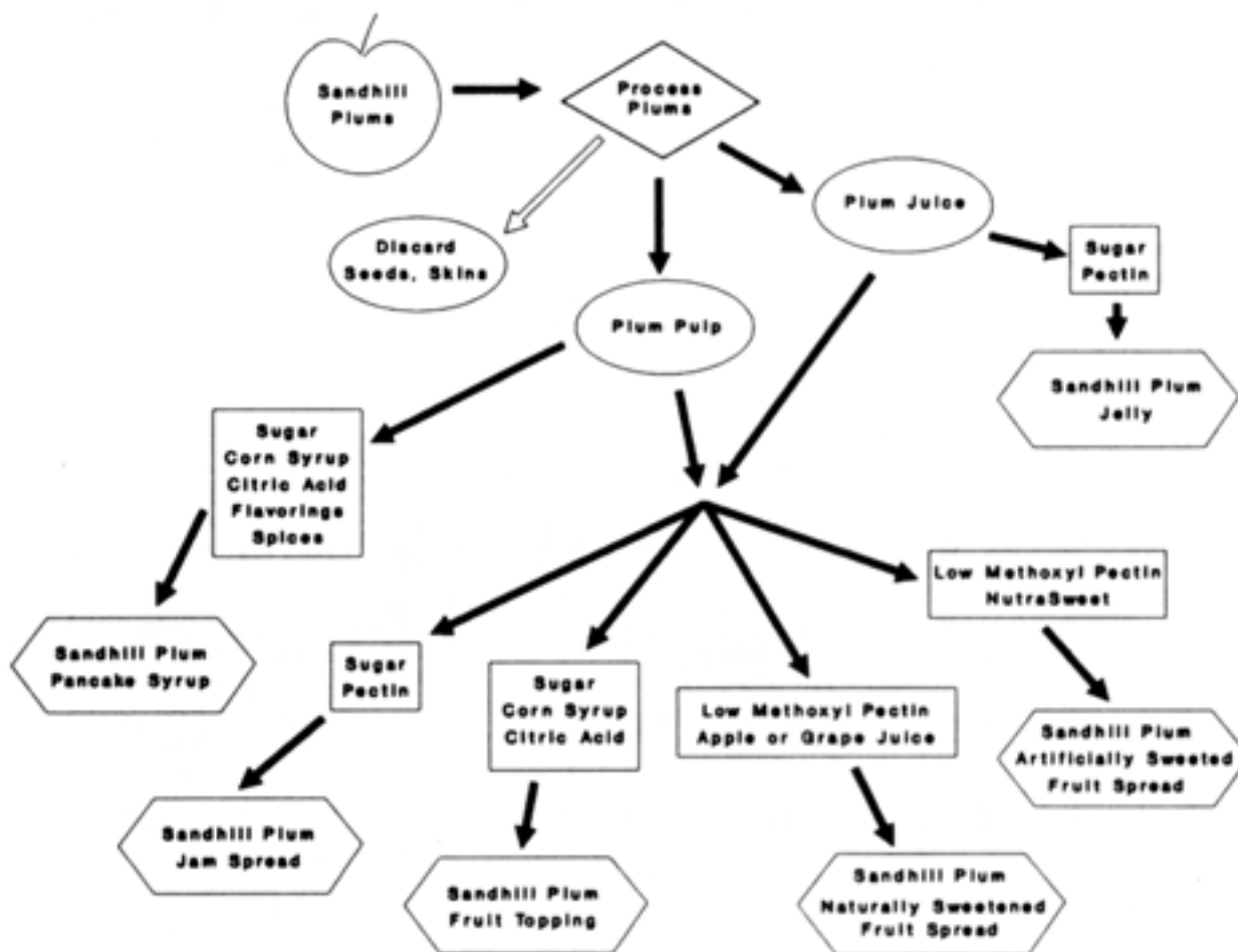
Fig. 5. A flow diagram for the manufacturing process of six sandhill plum products currently being produced in Kansas. Items enclosed in an oval represent ingredients derived from the sandhill plum. Additional ingredients are enclosed in rectangles, and final products are enclosed in hexagons.
