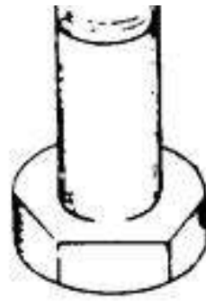
Fig. 2-16. Detail of the standoffs for the bottom plate of the filter unit.
