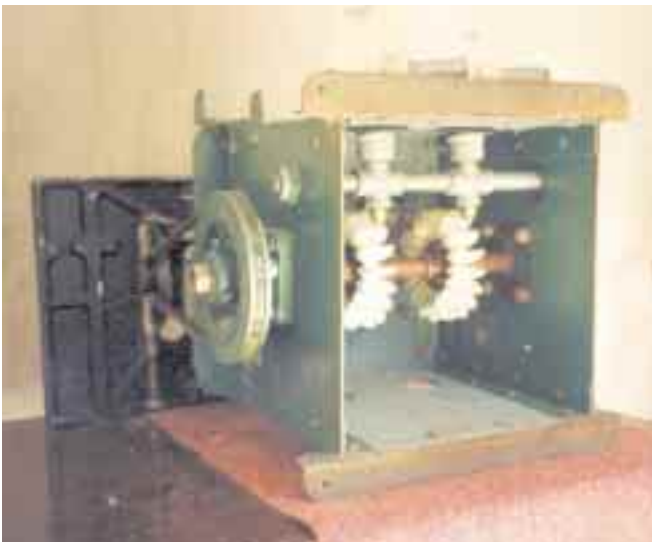
The Watermotor on its side with twin turbines exposed.
