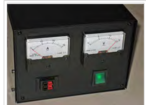
A simple desktop power supply with power output connector seen at lower-left and power input connector (not shown) located at the rear
