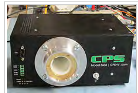
A 30 kV high voltage power supply with Federal Standard connector, used in electron microscopes
