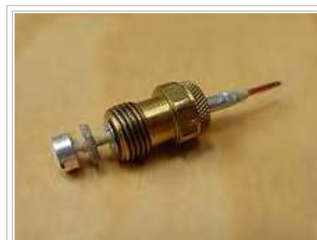
Thermocouple connection in gas appliances. The end ball (contact) on the left is insulated from the fitting by an insulating washer. The thermocouple line consists of copper wire, insulator and outer metal (usually copper) sheath which is also used as ground. [23]
