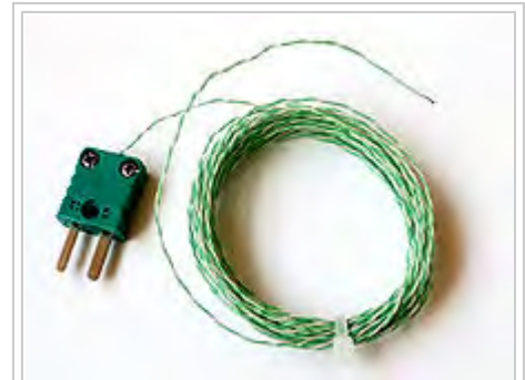
Typical low cost type K thermocouple (with standard type K connector). While the wires can survive and function at high temperatures, the plastic insulation will start to break down at 300 °C.
