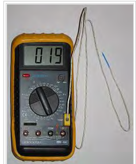
Thermocouple connected to a multimeter displaying room temperature in °C
