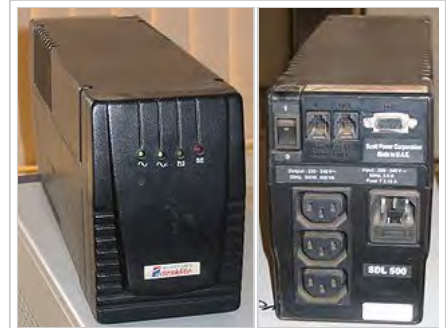
A small free-standing UPS with one IEC 60320 C14 input and three C13 outputs
