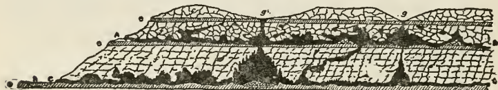
Fig. 188.—Cross section of cavern A B, upper gallery (ancient); g g, sink-holes; C D, lower gallery (modern); h, stream; A, old mouth of cavern; f f f, limestone; C, present mouth of cavern; e e e, hard rock
