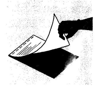
8 Hook the stencil with the backing paper attached on to the metal clips on the stencil drum
