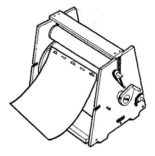
10 Remove the handle from the stencil drum and attach the pressure roller handle to the pressure roller
