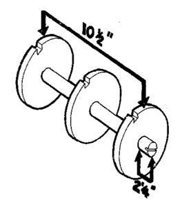
5 Make a U shaped piece of hardwood, like that shown in the drawing, 10%" long and %" thick. This should fit in the wooden discs as shown. Join to the discs with screws
