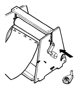
through the stencil turn the pressure roller anti-clockwise. If not enough ink is passing through the stencil add extra rubber bands or rub your fingers over the backing paper to squeeze the ink through. Once this is done the ink will flow continuously
