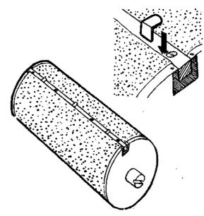
9 Cut out two washers from a plastic bottle or something similar. Put one on each end of the drum shaft to allow the stencil drum to turn freely
