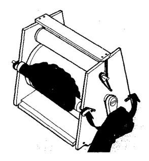
6 Remove the inking roller and store it in the back of the duplicator
