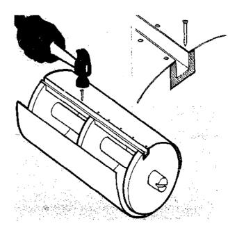
7 Cover the stencil drum with felt or absorbent material, allowing the material to overlap. Cut out the fabric grip from a strip of hardwood %6" square and 10%" long. Put the fabric grip into the channel on the stencil drum. This will tighten the fabric around the drum. Trim as required then secure the fabric grip to the stencil drum with screws
