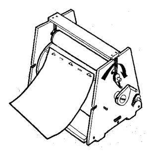
9 Put the pressure roller into the working position
