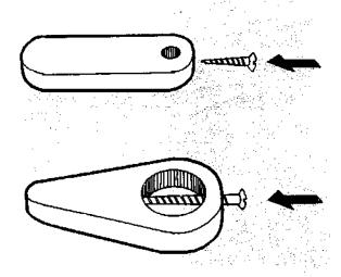
To attach the handles to the shafts put a screw of minimum length 1½" through the end of the handle
