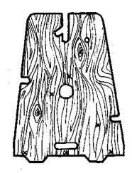
2 Using template 3 cut out the base from %" thick planed wood and make a groove %" deep for inserting the deflector plate (item 4)
