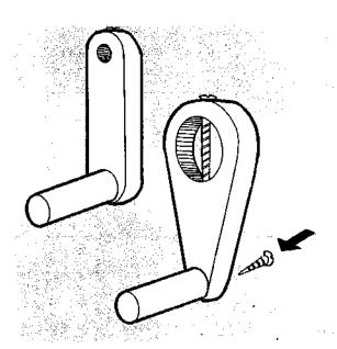
3 Join a length of dowel to the handle and attach it using a countersunk headed screw
