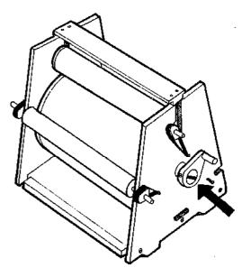
4 Put the ink along the roller in the trough between the roller and drum.
