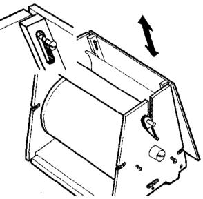
3 The top cover panel (item 13) should fit underneath the case handle (item 7)
