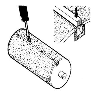
Attach three metal grips to hold the stencil. These grips should be positioned in such a way that the head of the stencil you use will be held in position (different stencils have different head fittings).
