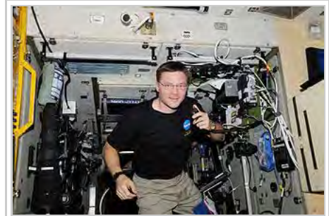
NASA astronaut Col. Doug Wheelock, KF5BOC, Expedition 24 flight engineer, operates the NA1SS ham radio station in the Zvezda Service Module of the International Space Station. Equipment is a Kenwood TM-D700E transceiver.
