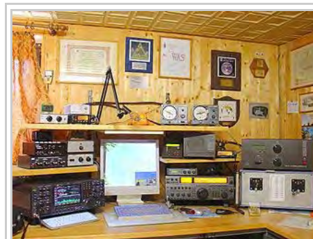
An example of an amateur radio station with four transceivers, amplifiers, and a computer for logging and for digital modes. On the wall are examples of various amateur radio awards, certificates, and a reception report card (QSL card) from a foreign amateur station.
