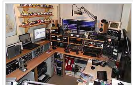
An amateur radio station in the United Kingdom. Multiple transceivers are employed for different bands and modes. Computers are used for control, datamodes, SDR and logging.
