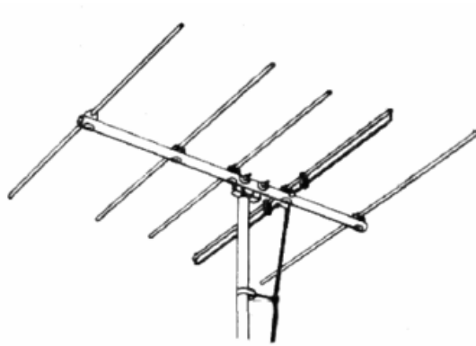
Yagi-Uda television antenna for analog channels 2-4, 47-68 MHz
