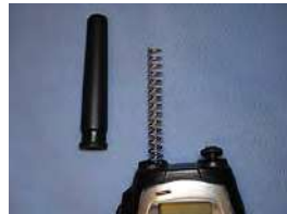
Rubber Ducky antenna on UHF 446 MHz walkie talkie with rubber cover removed.
