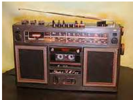
Quarter-wave whip antenna on an FM radio for 88-108 MHz
