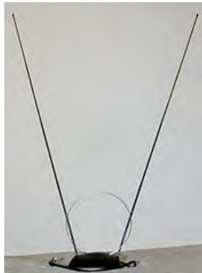
"Rabbit ears" dipole variant for VHF television reception
