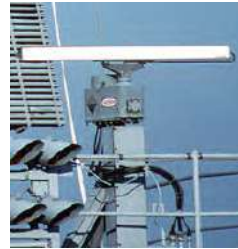
X band marine radar slot antenna on ship, 8 – 12 GHz.
