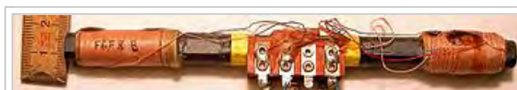
Loopstick antenna from an AM broadcast radio, about 4 in (10 cm) long. The antenna is inductive and, in conjunction with a variable capacitor, forms the tuned circuit at the input stage of the receiver.
