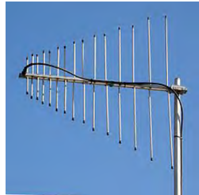
Log-periodic dipole array covering 140-470 MHz
