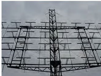
108 MHz reflective array antenna of AN-270 radar used during WW2.
