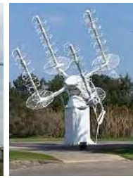
Array of four axial-mode helical antennas used for satellite tracking, France
