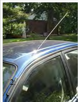
Whip antenna on car, common example of an omnidirectional antenna
