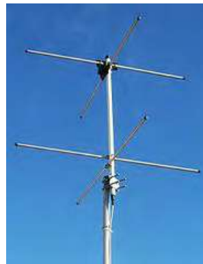
Two-element turnstile antenna for reception of weather satellite data, 137 MHz. Has circular polarization.
