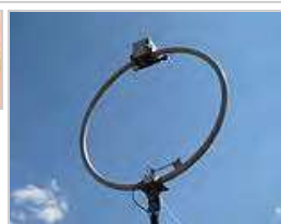
Loop antenna for transmitting at high frequencies, 2m diameter
