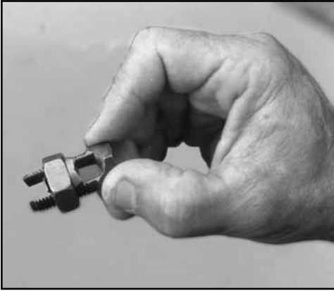
Use a stainless steel hose clamp or brass kearny nut to make your connection.
