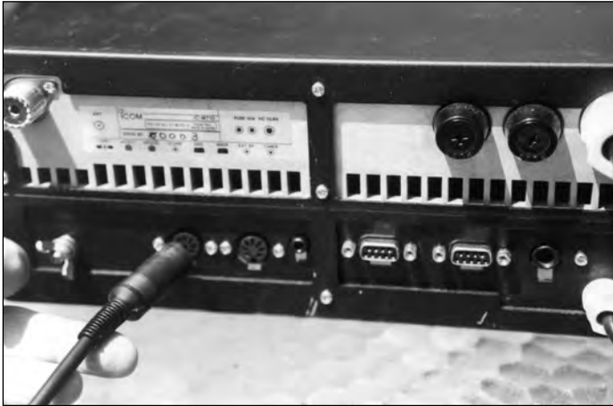
Marine SSB will accept the radio modem and computer on rear accessory plugs.
