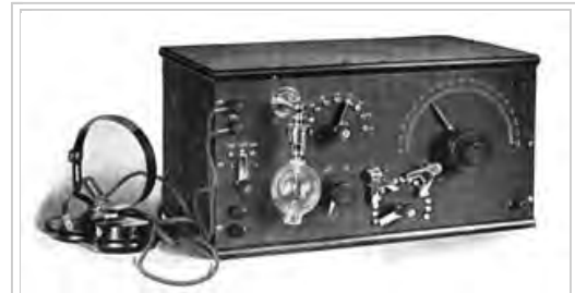
De Forest's first commercial Audion receiver, the RJ6 which came out in 1914. The Audion tube was always mounted upside down, with its delicate filament loop hanging down, so it did not sag and touch the other electrodes in the tube.
