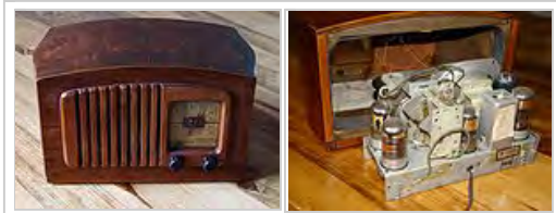
During the 1940s the vacuum tube superheterodyne receiver was refined into a cheap-to-manufacture form called the "All American Five" because it only required 5 tubes, which was used in almost all broadcast radios until the end of the tube era in the 1970s.
