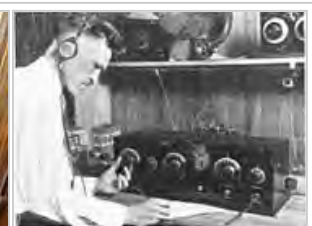
Tuning a Neutrodyne TRF receiver with 3 tuned circuits ( large knobs )
