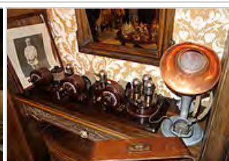
Atwater-Kent TRF receiver from the 1920s with 2 RF stages ( left ), detector and two audio amplifier tubes ( right ). The loudspeaker consists of an earphone coupled to an acoustic horn which amplifies the sound.
