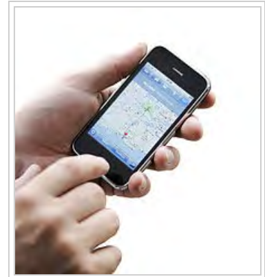
A modern smartphone has several digital radio transmitters and receivers to connect to different devices; a cellular receiver, a wireless modem, a bluetooth modem, and a GPS receiver
