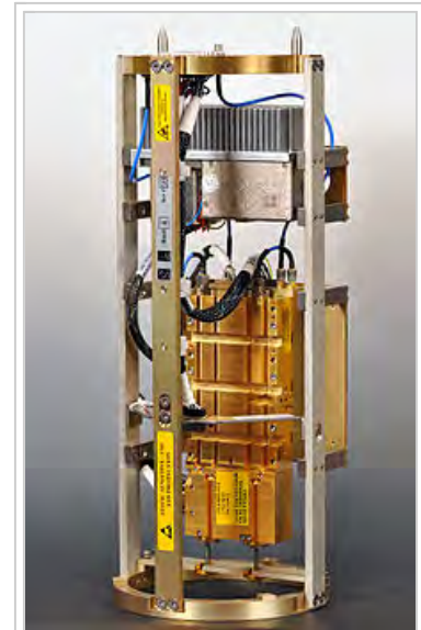
ALMA's Band 5 receivers detect electromagnetic radiation with wavelengths between about 1.4 and 1.8 mm (211 and 163 GHz). [2] The picture shows only peripheric components of the receiver such as the Local Oscillator multiplier chain. The main receiver components of the ALMA band 5 receiver, such as horn antennae, superconductive SIS mixers, and cryogenic low-noise amplifiers, reside on a cartridge that is inserted into a cryostat and cooled to 4K, 12K, and 90K, respectively
