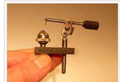
A galena cat's whisker detector from a 1920s crystal radio
