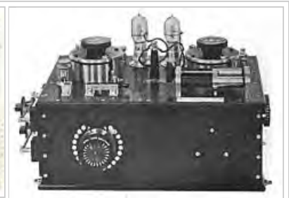
Marconi valve receiver for use on ships had two Fleming valves ( top ) in case one burned out. It was used on the RMS Titanic .
