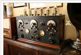
Early 6 tube TRF receiver from around 1920. The 3 large knobs adjust the 3 tuned circuits to tune in stations
