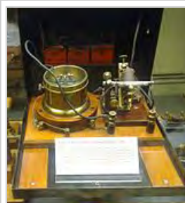
One of Marconi's first coherer receivers, used in his "black box" demonstration at Toynbee Hall, London, 1896. The coherer is at right, with the "tapper" just behind it, The relay is at left, batteries are in background
