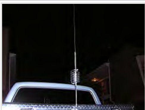
Typical center-loaded mobile CB antenna. Note the loading coil, which shortens the antenna's overall length.
