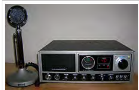
Typical 1980s CB base station, used with outdoor antenna. This radio may also be used in an automobile, since it is powered by 13.8V DC. Shown with Astatic Power D-104 desk mic
