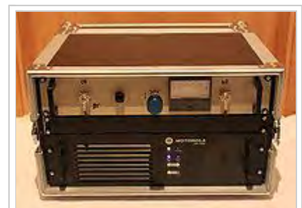
Motorola MOTOTRBO Repeater DR3000 with duplexer mounted in Flightcase, 100% Duty cycle up to 40 W output
