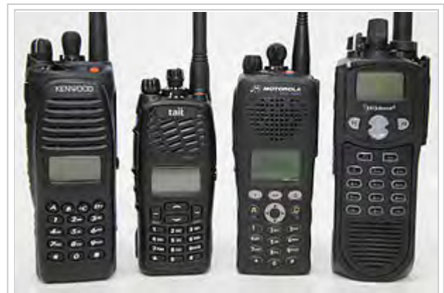
Several modern two-way hand-held radios compatible with the Project 25 digital radio standard (Mobile and base station radios not shown)
