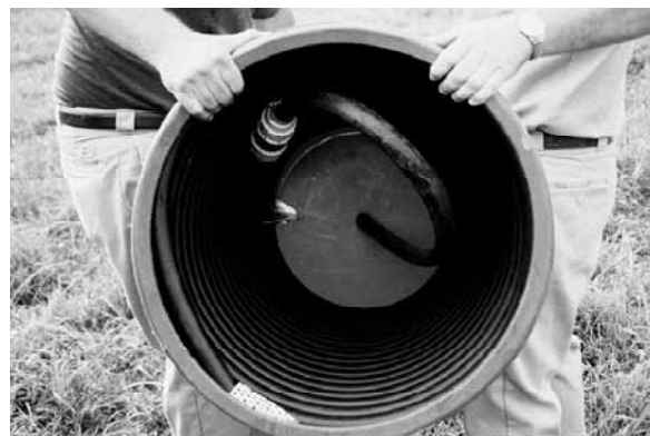
Figure 11. Inside of Sling Pump
