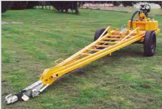
Ready for towing: The folded tripod in trailer mode will carry 60 metres of 3m (10-ft) drill pipe in racks
