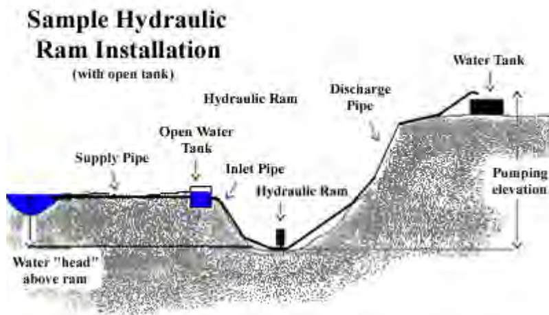
Figure 2. This installation is one option used where the inlet pipe is longer than the maximum length allowed. The open water tank is required to allow dissipation of the water hammer shock wave.
