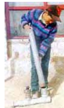
Prototype ram pump in India -- built for one-tenth the commercial price
