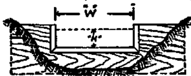
WEIR TABLE FOR DETERMINING THE FLOW OF STREAM
