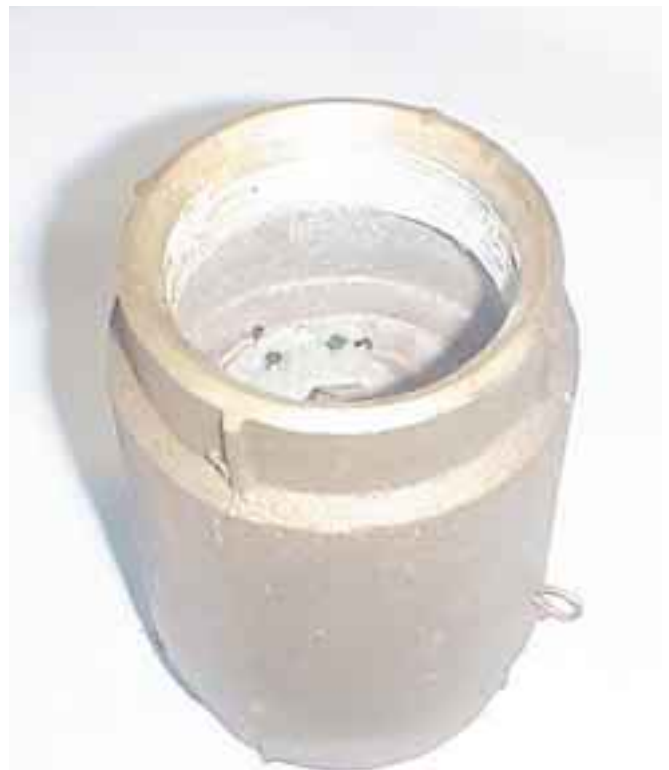
The check valve with the wire poking out of the air sniffer hole.
