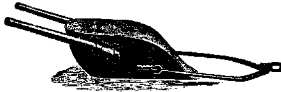
Figure 27. Steel scoop scraper used in North America in the nineteenth century
