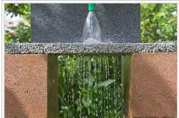
Permeable paving demonstration
