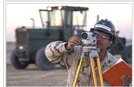
Surveyor at work with a leveling instrument
