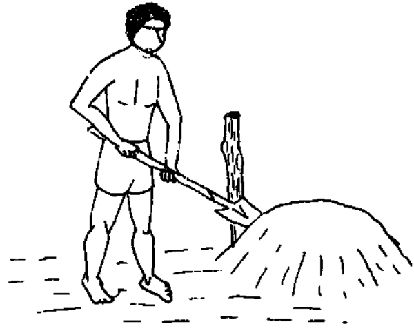
Fill to the top of this peg.
