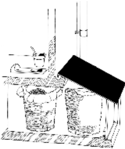
Figure 4.10 A single-vault, solar-heated eco-toilet with moveable containers, in this case two large baskets. When the first basket is full it is placed directly under the solar heater and remains there until the second basket is full.
