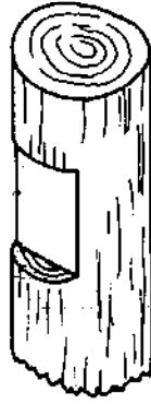
FIGURE 53 ROUND POLE NOTCHED FOR SAWN FRAMING MEMBER.
