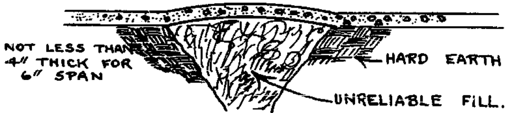
FIG. 98. SOLID CONCRETE FOOTING BRIDGE OVER FILLED EARTH
