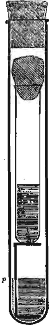
FIG. 9. Buchner tube for the anaerobic cultivation of bacteria: p , the alkaline pyrogallol solution; inner tube contains culture of organism (after Omeliansky).
