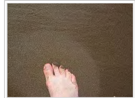
Foot pressing in soil causes soil to dilate, drawing water from the surface into the pores
