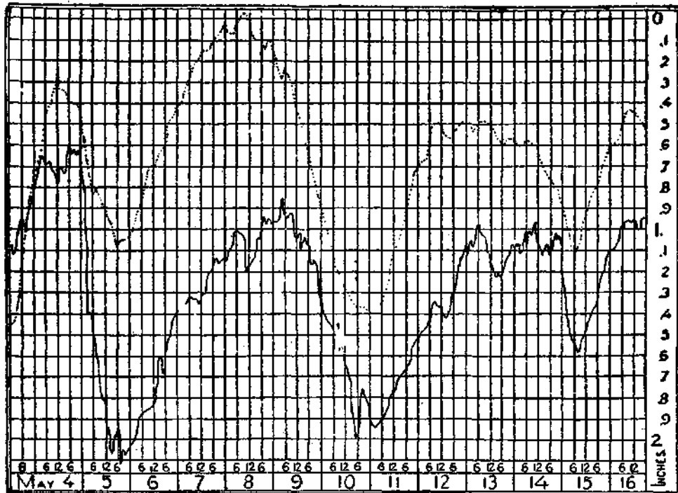
FIG. 36. — Showing fluctuations in the rate of flow of water from a spring at Whitewater, Wisconsin, May 4 to May 16, and the barograph record at Madison, Wisconsin, for the same period. Both reduced to natural scale. Heavy curve represents the spring.
