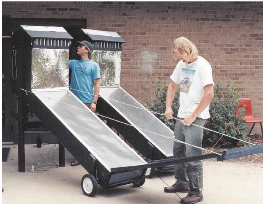
Above, Photo 4: Setting the front reflector angle.
