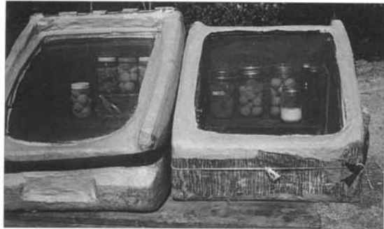
Solar cookers (eleven years old) in action (Ch. 10) bottling fruit and heating milk and coffee. Note curved (cracked windscreen) glasses and two-tier shelf to reach hottest part of stove. Hinge for reflector on stove left. Reflector not used.
