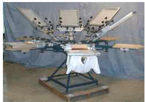
6 - color t-shirt & cap printing press. You do not need this to print solar cells, all you need is a flat and sturdy table top.
