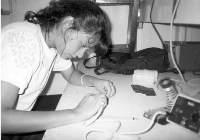
Above: Laying down traces.
