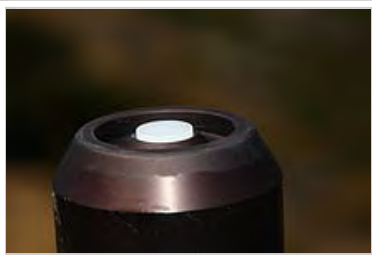
A Pyranometer, a component of a temporary remote meteorological station, measures insolation on Skagit Bay, Washington.
