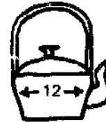
Figure 5.9. Fixing pot-hole size for a wide variety of pots. When different pots are to be used on one stove the most effective solution is to have the front pot-hole as large as the most commonly-used large pot, the second as big as the pot commonly used with the largest pot, and to use metal pot rings for the rest. Thus:
