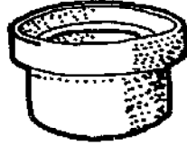
Figure 5.7. Sunken pots. Shallow pots will be further away from the fuel unless concave metal pot rings are used. The lower drawing shows a special pot with raised pot rim for easier handling (Micuta, 1981, and others).
