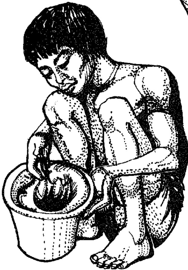
Figure 12.18. Moulding Thai stove liners.
