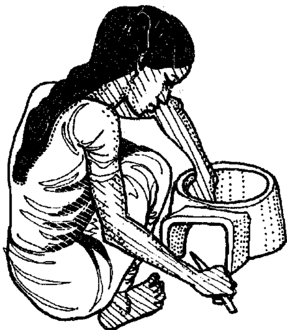
The firebox entrance is cut out
