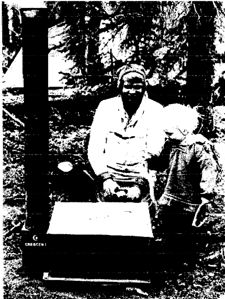
Figure 13.27—The author and his son light up the Three-Way Stove for the first time. Note how a tin can has been used as an elbow adapter for the stovepipe.
