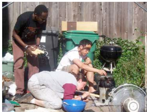
Figure 12: The team tends the unmodified stove during a mulah test with wind (note the fan in the lower right).
