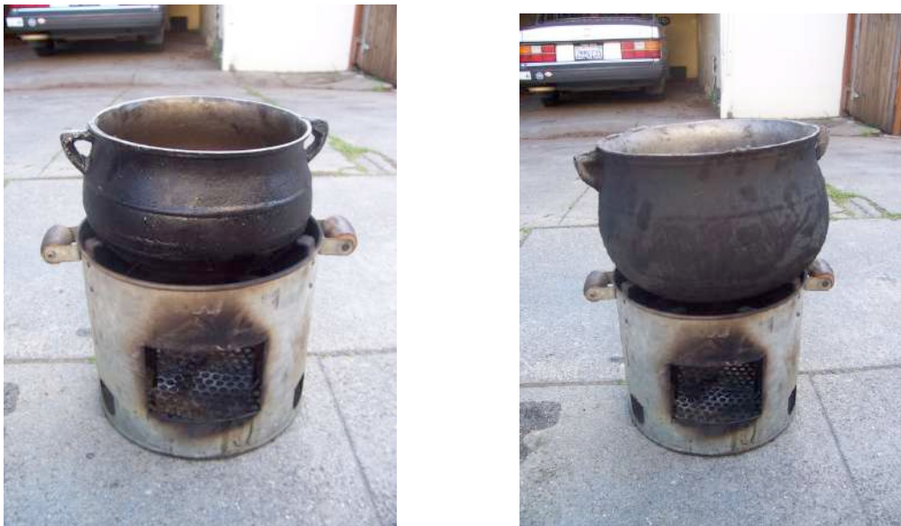
Figure 2: (Left) Small pot sitting on top of unmodified Tara stove. (Right) Large pot sitting on top of unmodified Tara stove.
