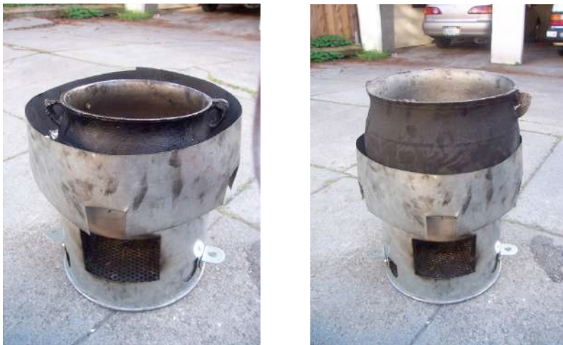
Figure 8: (Left) The modified Tara stove with the small traditional pot. Note how far it sinks into the stove. (Right) The modified stove with the large traditional pot. The wind collar effectively shields the large air gap that was present on the unmodified stove.
