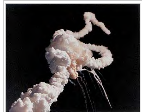
Space Shuttle Challenger was torn apart T+73 seconds after hot gases escaped the SRBs, causing the breakup of the Shuttle stack
