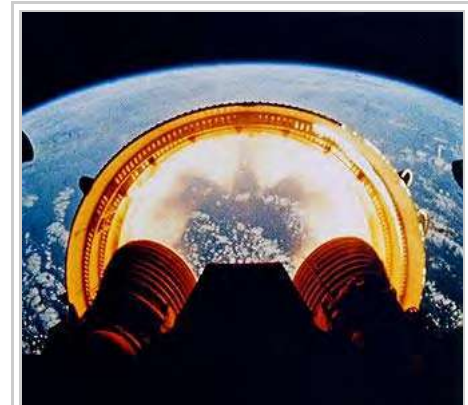
Apollo 6 while dropping the interstage ring
