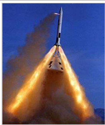
Apollo LES pad abort test with boilerplate crew module.
