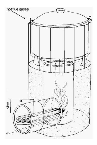
This picture shows a thin piece of metal (a skirt) wrapped around the pot. This skirt forces the hot flue gases to rub against the bottom and the <u>sides</u> of the pots. The gap between the pot and the skirt should be about 1cm (assuming you are using an average-sized pot). In our tests, this simple heat exchanger (an old coffee can works well!) almost <u>doubles the efficiency of the rocket stove.</u>
