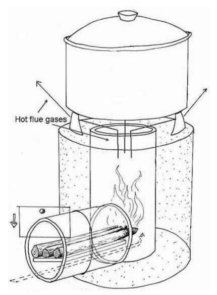
This elbow is then placed inside of a container that is filled with insulation. The container can be made from almost any material. We have used 5 gallon drums, brick, clay, cement. For insulation we suggest using wood ash or pearlite, or pumice,. Do <u>not</u> use massive things such as earth, sand, or cement. These will rob heat from the stove and reduce your combustion efficiency. For optimal use we recommend a 9" chimney and a 4" fuel feed magazine.
