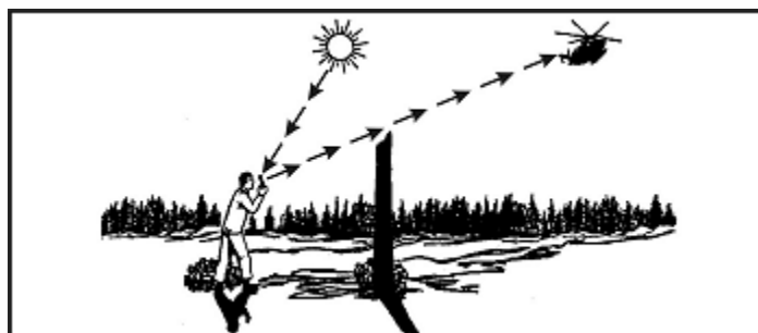
Figure 19-4. Aiming an Improvised Signal Mirror
