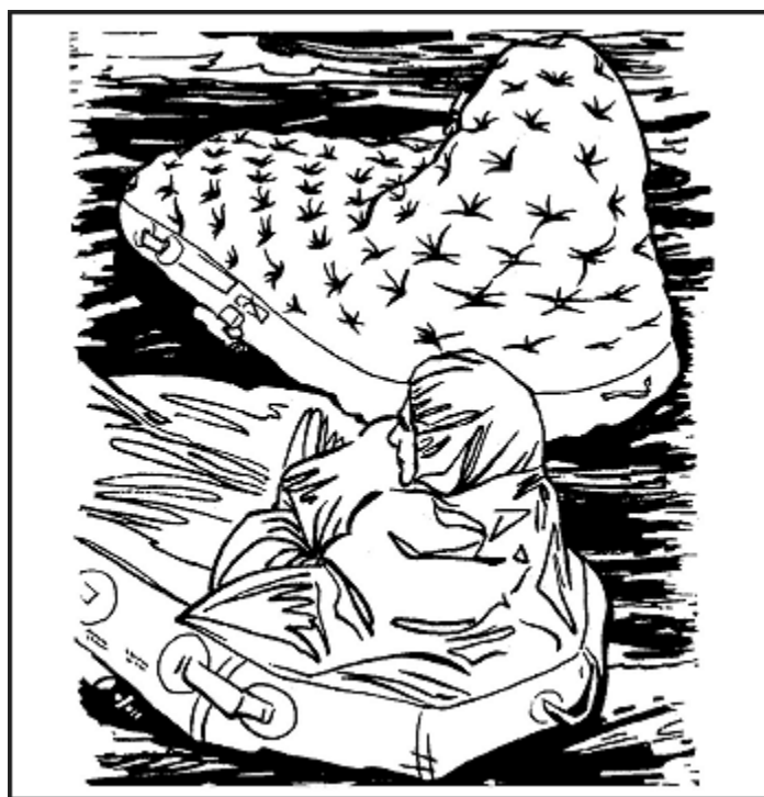
Figure 16-11. One-Man Raft With Spray Shield Inflated
