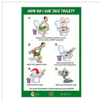
Instructions on using a urine-diverting dry toilet
