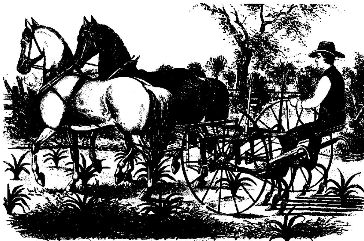
Combination riding and walking cultivators were popular during the late nineteenth century. On this model, the levers regulated the depth of the shovels. When the farmer rode the cultivator, he used his feet to guide the shovels down the crop row.
