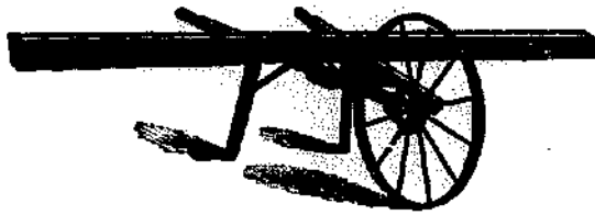
The wheelbarrow seeder dropped the grain from the seed box as the wheel turned. Then, the seed had to be covered with a harrow.
