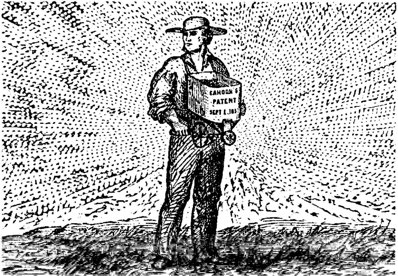
Prior to the perfection of the grain drill, farmers either seeded their crop by hand or they used a broadcast seeder. The handcrank broadcast seeder consisted of a bag with a star-shaped disk at the bottom. As the crank turned, seed fell onto the spinning disk and scattered across the furrows. (Smithsonian Institution.)
