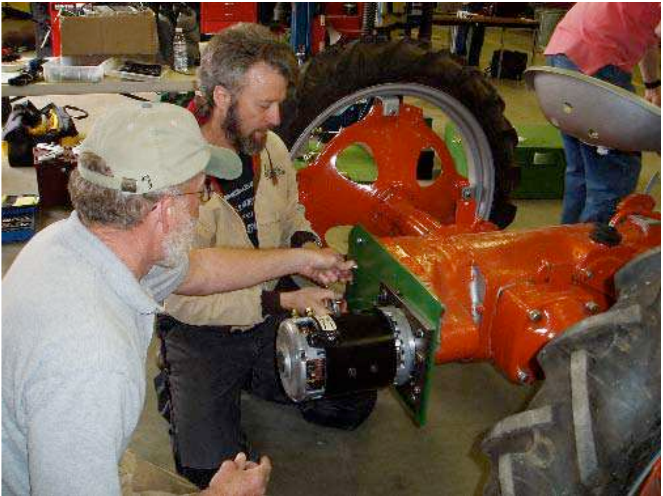
Motor plate installation.
