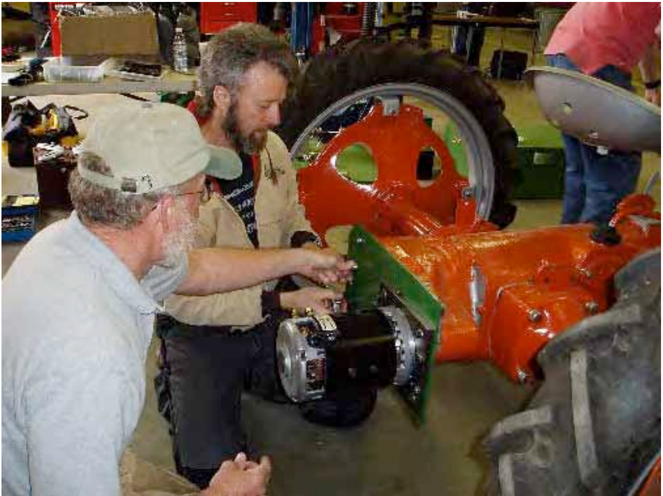
Motor plate installation.
