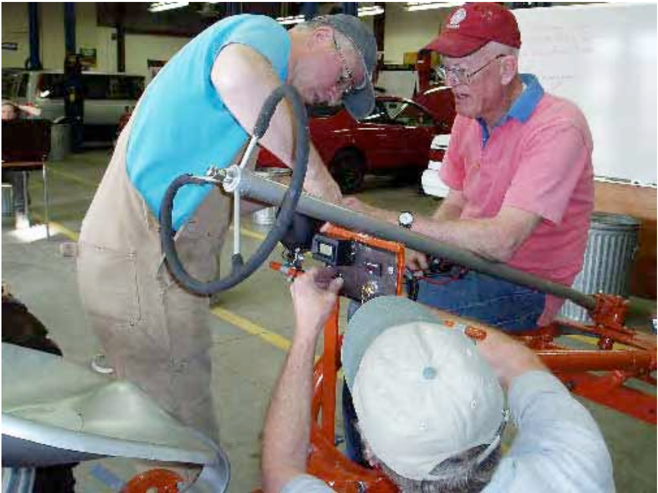
Instrument cluster installation.
