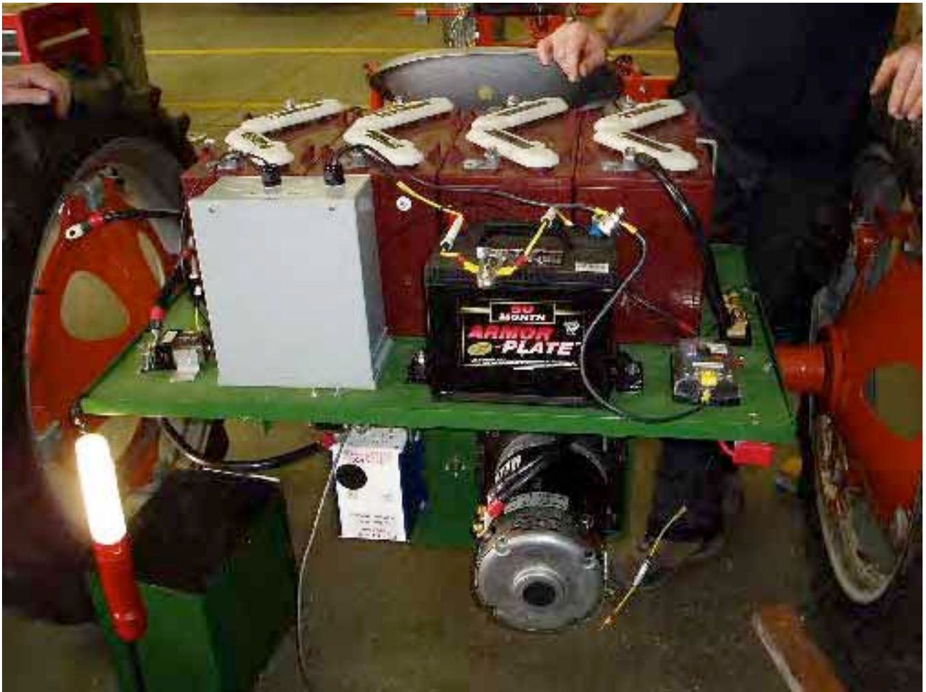
Battery rack and battery bank installation.
