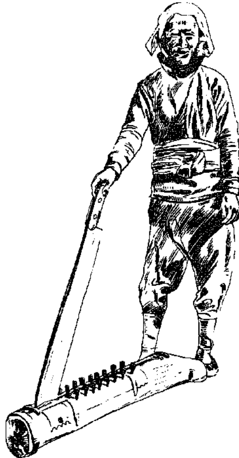
FIGURE 106. - Chinese straw cutter (Shansi Province, Mainland China), with iron teeth to prevent straw slipping.
