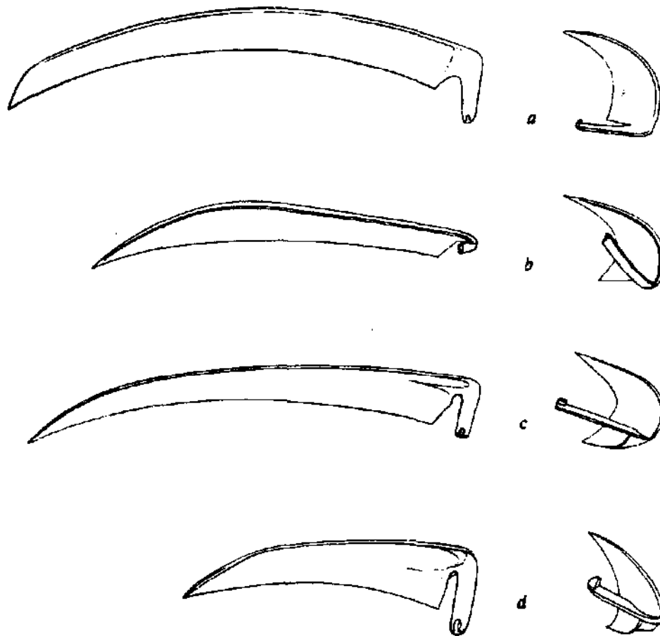
FIGURE 86. - Scythe blades: (a) ground blade from the U.S.A.; (b) scythette blade; (c) hammered Austrian blade; (d) short, heavy blade for weed and brush cutting.
