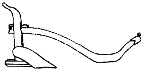
FIGURE 42. - Kedah plough (Malaysia) with improved share design.
