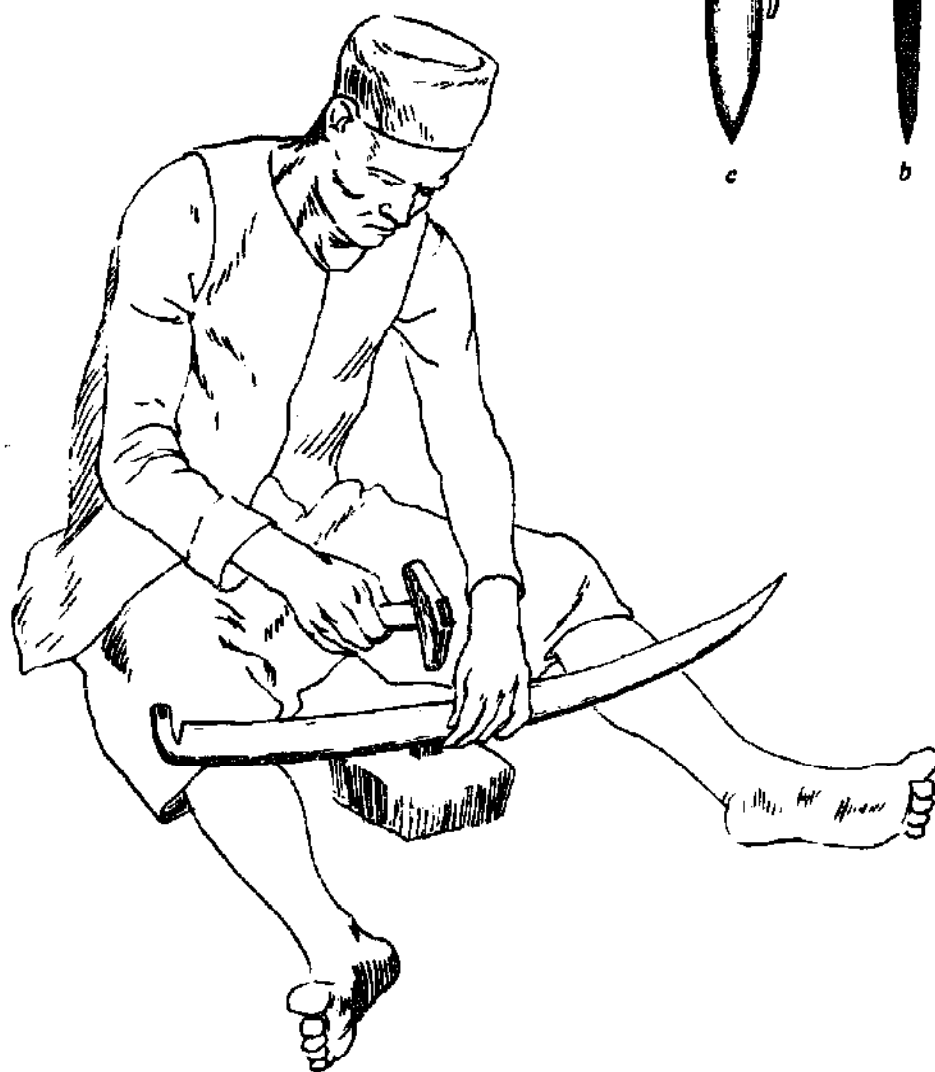
FIGURE 91. - Farmer hammering a scythe blade.
