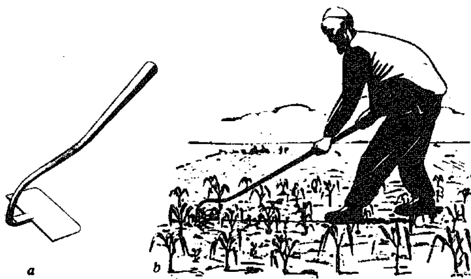
FIGURE 77. - Chinese pulling hoe: (a) blade and long iron hoe socket; (b) work with the hoe.
