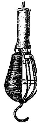
Fig. 28—For work on farm machinery on darker days, an extension cord with lamp reflector and bulb protector is most useful shop equipment.
