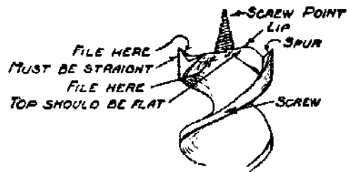
Fig. 17—Parts of an Auger Bit and where to file.
