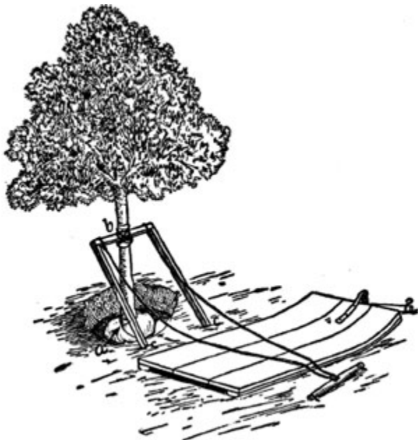
RIG FOR MOVING TREE
