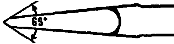
Fig. 5.28. Cold chisels are ground to an angle of 65 degrees for average work.
