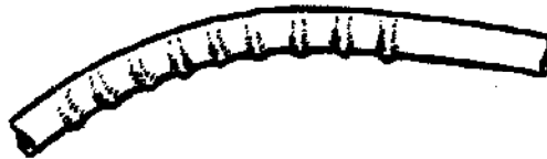
Fig. 13.30. Wrinkle bending larger diameter pipe.
