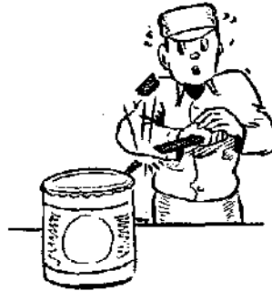
Fig. 2.14. A file is not made for prying. Always select the correct tool for the job.
