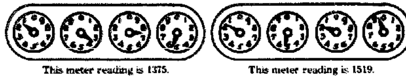
Fig. 37.2. Reading a meter. "The reading on the second dial from the right, although the hand is at number 2 should be read as number 1 until the hand which moves clockwise on the first dial has passed zero. To determine the amount of electricity used in one month, read the meter on the same day each month and subtract the preceding month's reading: 1519 - 1375 = 144 kilowatt hours. The outside meter mounted on the house should preferably be placed on the back porch or near the rear of the structure, where it will not detract from the appearance of the house but may be conveniently read." (From J. B. Kelly, Ida C. Hagman, and Earl G. Welch, "Electric Service for the Farmstead," College of Agriculture, University of Kentucky, Extension Circular 311, pp. 11-12.)
