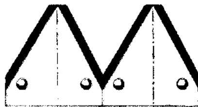
New sections—proper bevel and angle for good work
