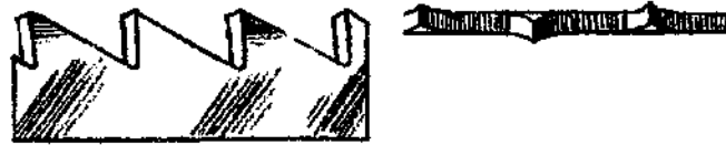
Fig. 5.13. Views of a section of a rip saw which has been correctly filed and set. Note there is no bevel on the front of the teeth. The teeth are filed straight across.
