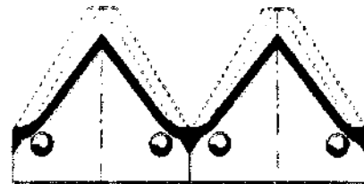
Improperly ground sections—narrow bevel and wrong angle which changes the angle of shear.
