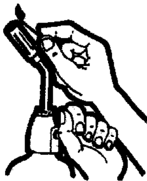
Fig. 18.3. Lighting a propane torch.
